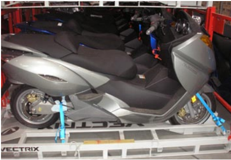
Representative tie down - front and back.
