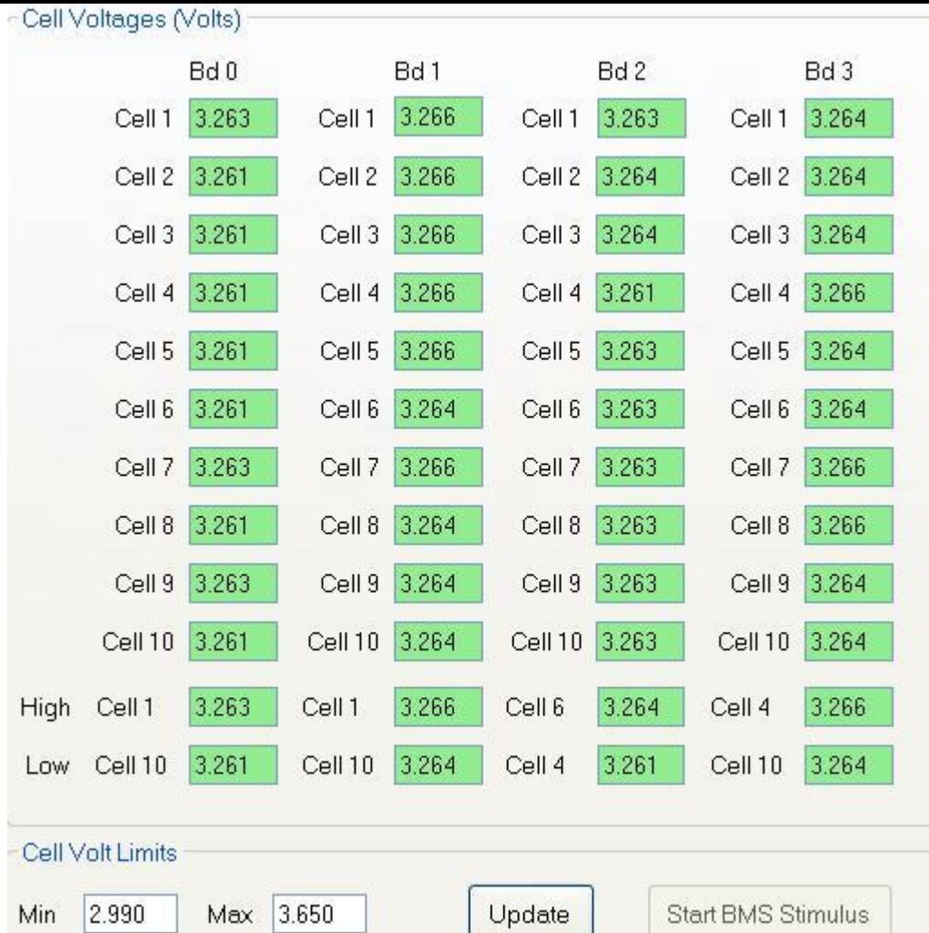
Figure 11 BMS Battery Cell voltage
